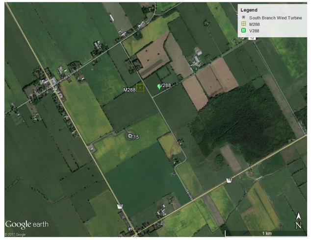
Measurement equipment at Location 3 was placed on the adjacent field to vacant lot receptor V288, facing the nearest turbine T15 (596m from the turbine). Location 3 was chosen to represent V288 due to setup limitations.
