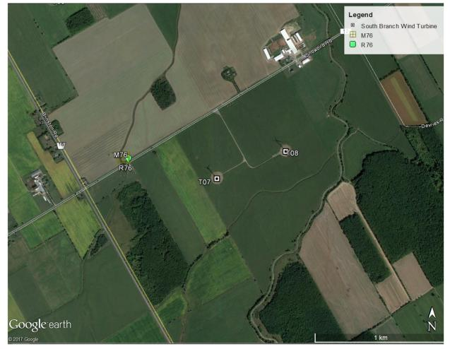
Measurement equipment at Location 2 was placed across the street opposite to the property of Receptor R76 identified in the Acoustic Assessment Report, facing the nearest turbine T07 (708m from the turbine). Location 2 is also close to turbine T08.
