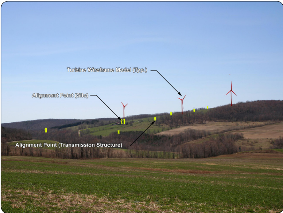
These data are superimposed over photographs from each of the viewpoints, and minor camera changes are made to align all known reference points within the view.
