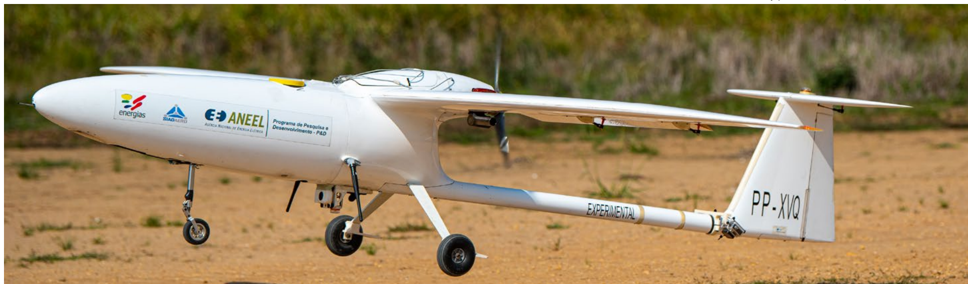
Remotely piloted aircraft (RPAs) for network monitoring.
