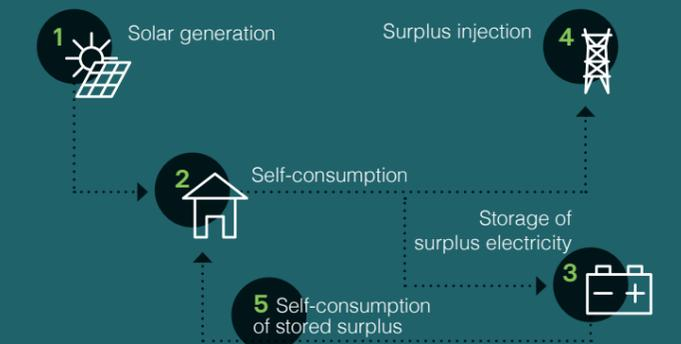
The solar power plant will produce electricity to be used on site, stored, or injected into the grid, depending on consumption needs.
